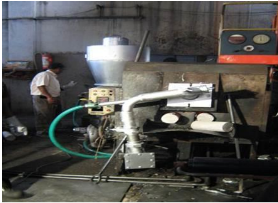
Aluminum Billet Heating for extrusion of sections.
