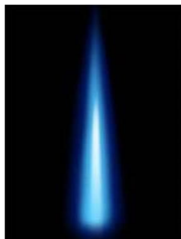
Blue Flame= Complete Combustion
