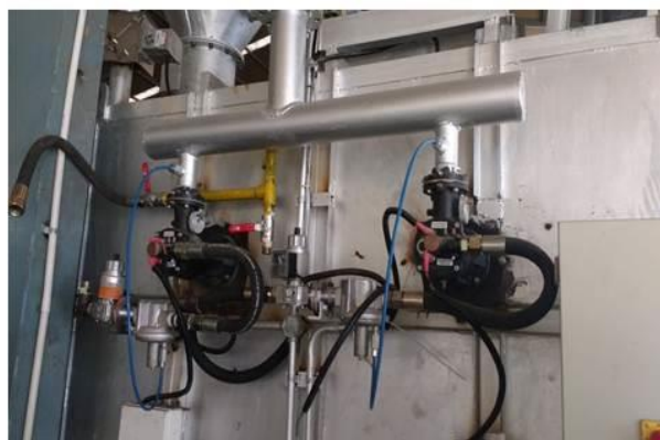
After: EE High velocity burners
